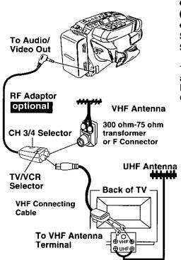
If TV has no VIDEO/AUDIO IN jacks, connect PV-RF16 RF Adaptor (optional, page 76). Tune TV to CH 3 or 4 to match RF Adaptor CH 3/4 Selector. Set Adaptor's TV/VCR Selector to VCR for playback.
