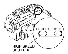
Press <u>HIGH SPEED SHUTTER</u> while recording.
